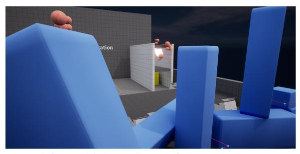
Fig. 1.1 The first example level in Unreal Engine 5. On the screenshot we can see blue dynamic obstacles, and pink flying pawns navigating to the bright target where they end their journey. The blue obstacles can be moved, and the graph regenerates around them, allowing the pawns to avoid them.
