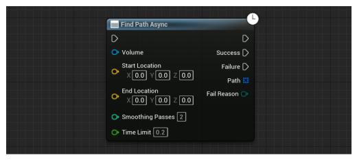
Fig. 3.5 Find Path Async node in a blueprint
